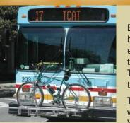
Every bus in the TCAT fleet has a bicycle rack mounted on its front end. These racks can help cyclists tame the hills and weather of Tompkins County. There is no additional fare for using the bike racks. TCAT is an innovator. In 1996, TCAT was the first bus system in New
